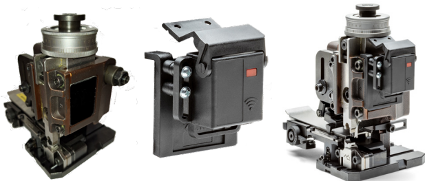
Figure 9: example of sensor installation on a generic applicator from the market
